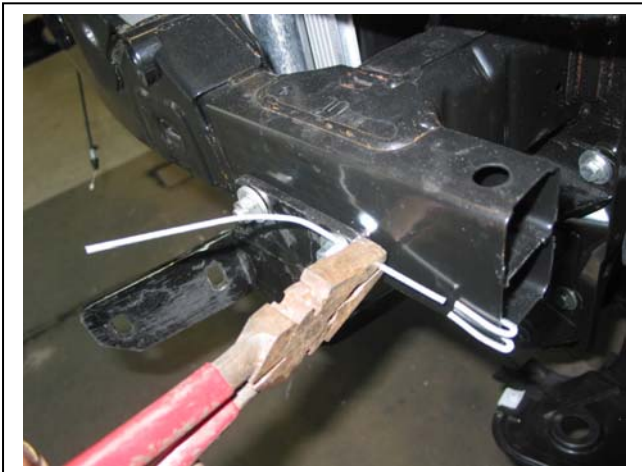
Figure 11 - Wiring trimmed and crimped to bumper support to stop possible rattle.
